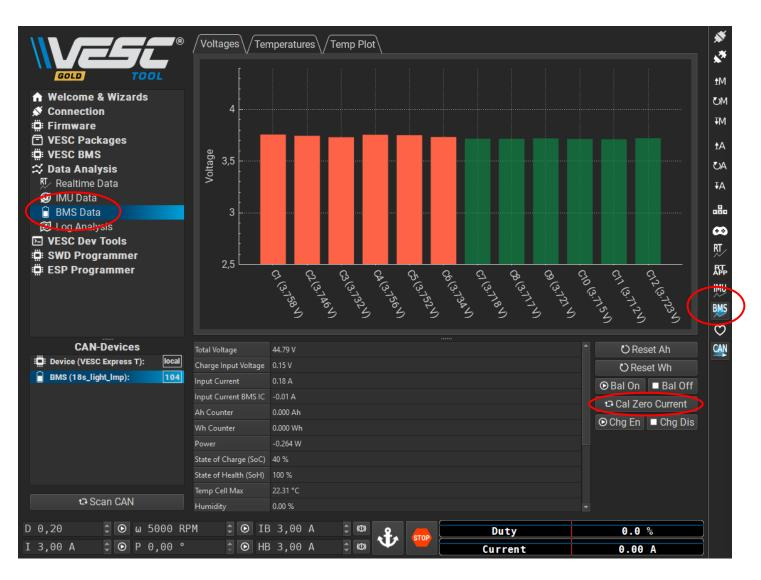
The next check is the temperature measurements. This window shows 7 temperatures. The temperature T1 and T2 are located on the BMS itself and show the temperture of the LTC chip and the Mosfet switch of the charge input. Temperature probe T1 on the BMS shows a T4 in this menu. T2 on the BMS shows as T3,T6,T7 and T3 shows as T5. Now plug your temperture probe(s) to T1, T2 or T3 on the BMS. These probes need to be an NTC10K with a beta value of 3380k.
