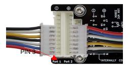
This example shows the balance connectors from two 6S batteries in series. The minus pole of the battery is connected to PIN 3. *First Cell Index* is set to 3
